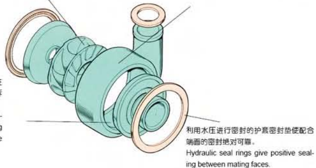
金属内衬配合端面具有一定的锥度，保证装配过程中精确对准，并保证部件易于拆卸或更换。 Mating faces in hard metal liners are tapered to allow positive alignment during assembly and allow components to be easily removed for replacement.
